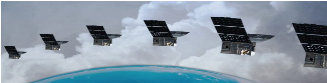
5 identical 6U small sats, each with an identical 5-channel radiometer, flying 5 minutes apart
