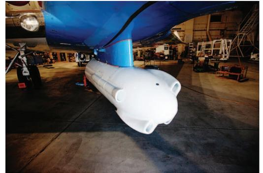
*Above, the UAVSAR (Uninhabited Aerial Vehicle Synthetic Aperture Radar) pod below the NASA Gulfstream III aircraft. Developed with ESTO funding, UAVSAR is now a fully-operational airborne instrument for surface deformation measurements. ESTO is currently conducting studies to integrate the technology onto the Global Hawk UAV platform. (Image Credit: Dave Bullock, Wired.com)*
