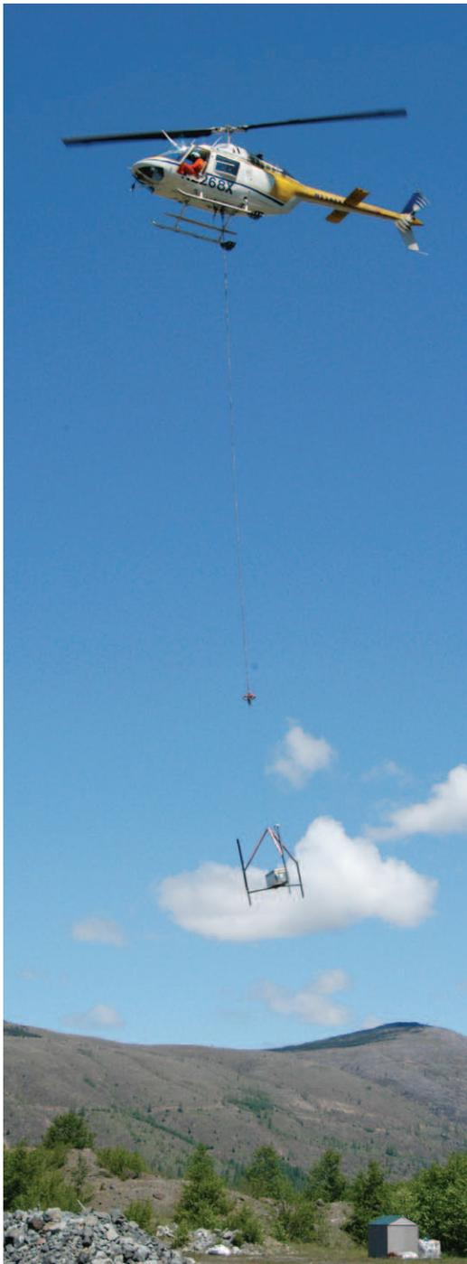
On July 14, 2009, several “spider” pods like the one shown above were lowered by cable from a helicopter hovering about 100 feet up and gently put in hot spots inside and around the volcano crater of Mt. St. Helens. (Image Credit: Willie Scott / USGS)
