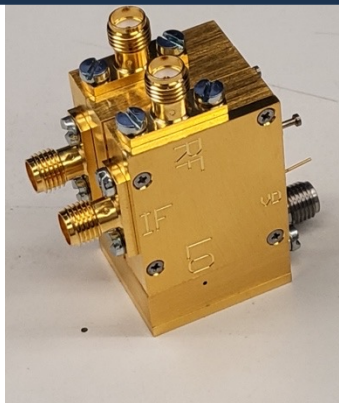
2 nd stage downconverter (12–18 GHz → 3–9 GHz)
