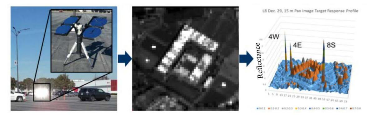
The study showed that small reproducible vicarious reference targets could be deployed as portable point sources for vicarious calibration at almost any location
