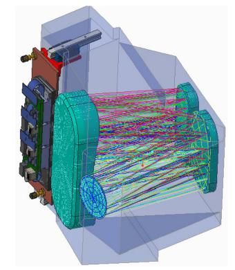
ATLIS-P is a testbed for future NASA and Raytheon funded demonstrations of calibration, VNIR and SWIR focal plane technology and any other technologies that support NASA and USGS SLI goals
