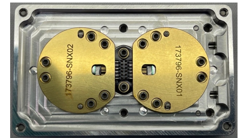
PBR-R Detector Engineering Model: 1.5" x 2.5"
