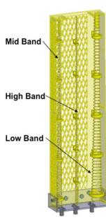
payload antenna (left) CubeRRT's includes 3 tapered helix elements to cover 6-40 GHz with gain 7 to 21 dBi in a 0.25U, 116g package
