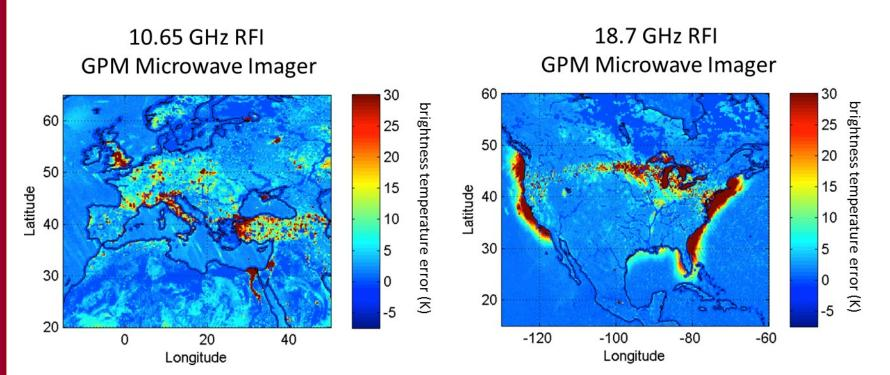
Images from NASA's GMI radiometer (above) at 10.65 and 18.7 GHz show the clear corrupting influence of RFI. Ideally, radiometers avoid RFI by operating in bands where transmission is prohibited. In practice, radiometers must co-exist with RFI sources due to shared spectrum allocations or operation in unprotected bands. Co-existence in some cases may be possible provided that a subsystem for mitigating RFI is included in future systems.
