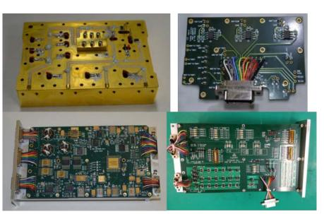
CubeRRT's RDB (below, ~ 0.25U, 170g, 10W) is the key technology, and is implemented using a Zyng 7100 COTS FPGA plus power and A/D components
