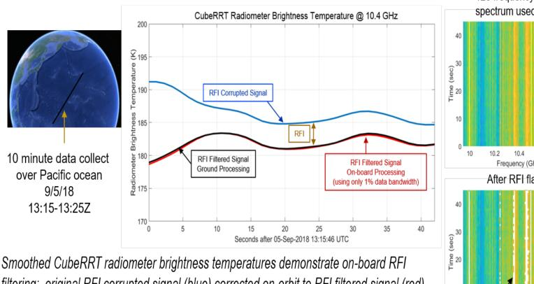
filtering: original RFI corrupted signal (blue) corrected on-orbit to RFI filtered signal (red) that is validated with ground processed data (black). On-board filtering requires 99% less data to be downlinked.
