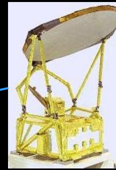
Advanced Microwave Scanning Radiometer (AMSR-E) MSFC/JAXA
