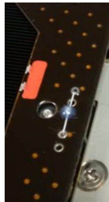
Intact tie-down after vibration testing
