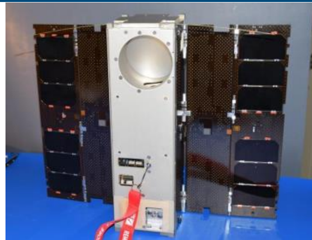
Fully Integrated Space Vehicle prior to final solar panel tie down
