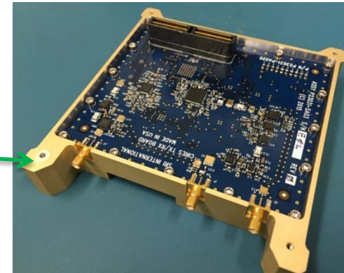
Tx/Rx Module: Includes: Tx and Rx RF analog chains, calibration loopback circuits, integrated ADC and DAC capability.
