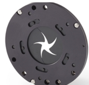
Shutter : successful endurance and thermo-vac
