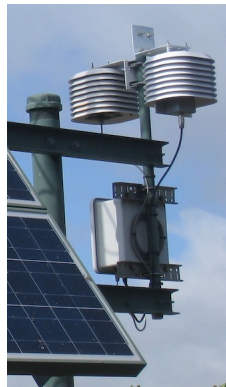
Meteorological Sensors (pressure, temperature)
