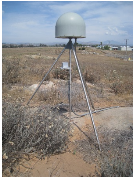
GPS Permanent station
