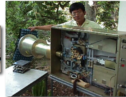
Outdoor testing of OSIRIS electronics & antenna Feed breadboards
