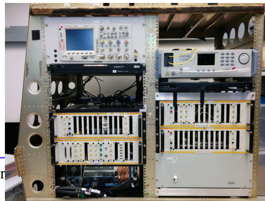
Step locked laser in DC-8 rack
