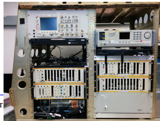
Step locked laser in DC-8 rack
