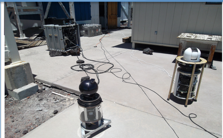
4STAR + AATS-14 calibration using Langley Extrapolation.
