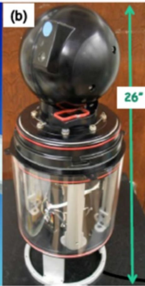
(a) Design for 4STAR tracking/scanning head and can. (b) Head and can as built. (c) 4STAR head on NASA C130 aircraft. (d) Rack and contents.
