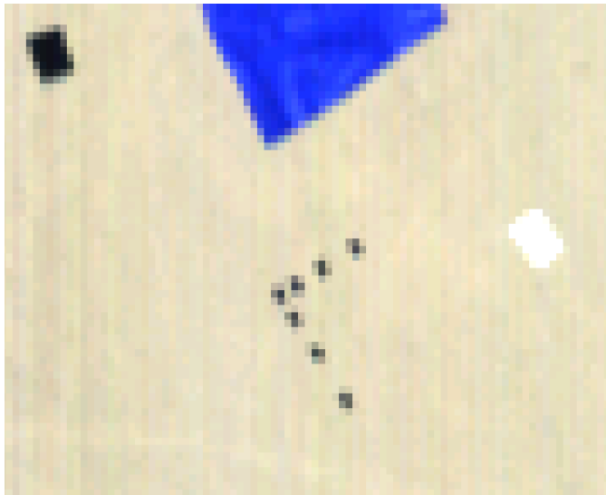
1' sq. targets placed 1' apart at corner, well resolved by PRISM
