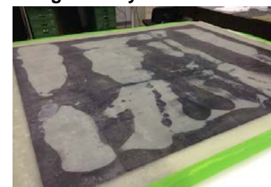
Full size radome fabricated using Wet Layout Process
