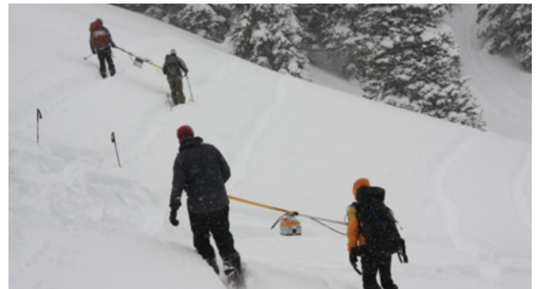
Snow depth measurement using FMCW Radar from skis and snowmobile
