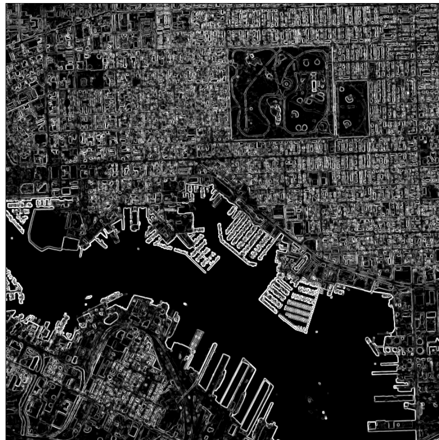
Frei-Chen edge difference operator result, maximum over spectral bands, thresholded at 0.07.
