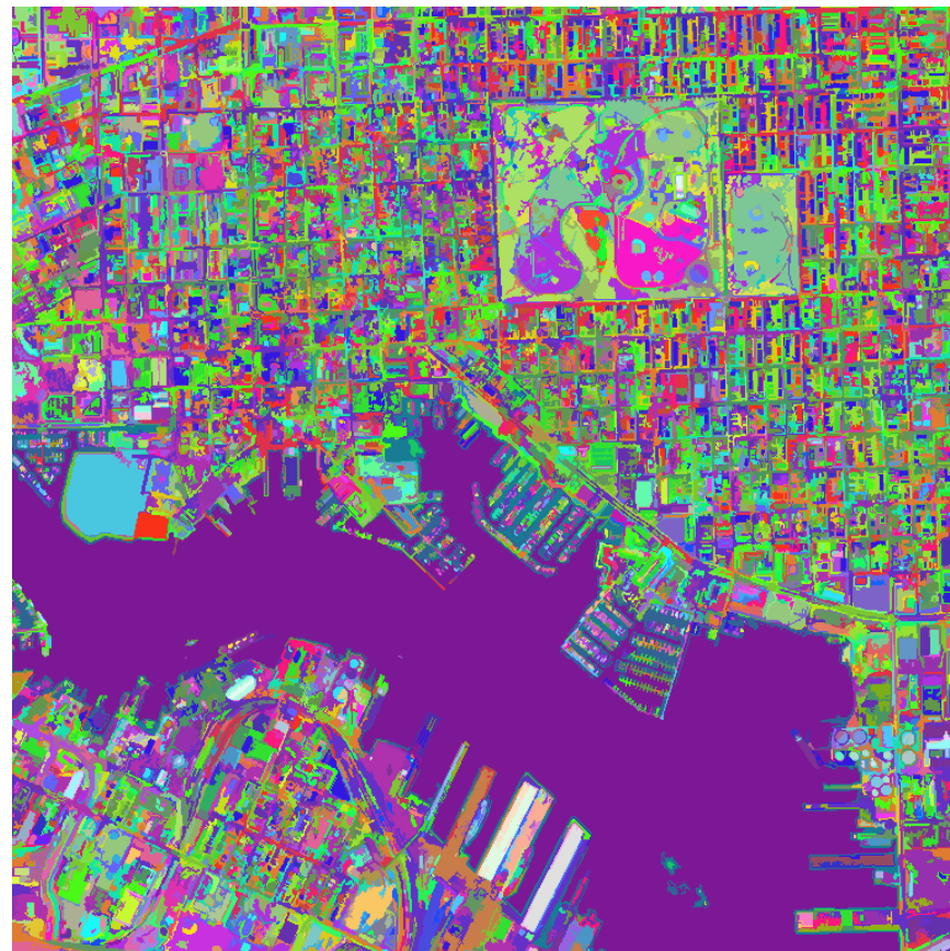
HSeg v. 1.61 result, E_t=0.05 and E_w=0.0 , at global dissimilarity 0.371, 192 region classes and 9954 region objects.
