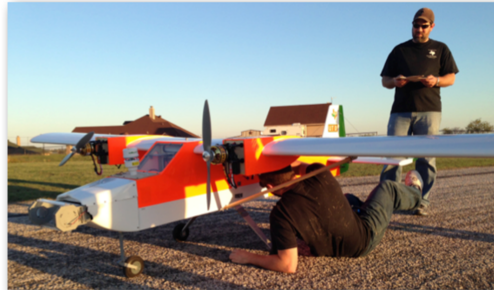
The model aircraft is equipped with a full suite of meteorological instruments for temperature, pressure, humidity, wind speed and direction as well as an EPA certified Grimm Model 1.109 Aerosol Spectrometer & 1.320 Nano Check which provides extremely precise size distributions within the size range 12 nm - T 32 μm in 43 size channels.
