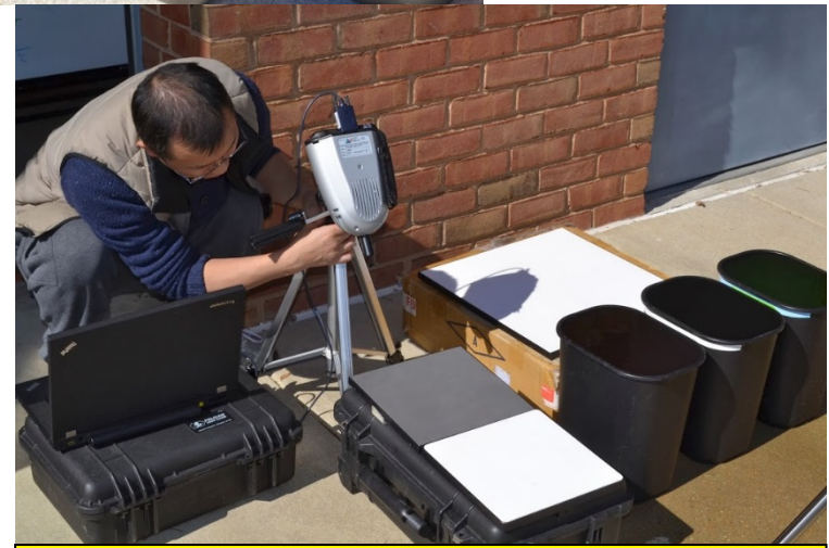
Measurements with spectrometer for calibration plates and algae
