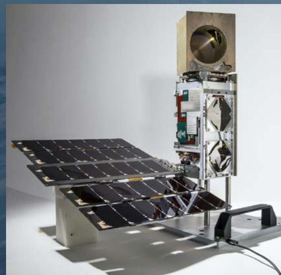
◀ TROPICS CubeSat Pathfinder with solar cell panel and radiometer. Credit: Blue Canyon Technologies
