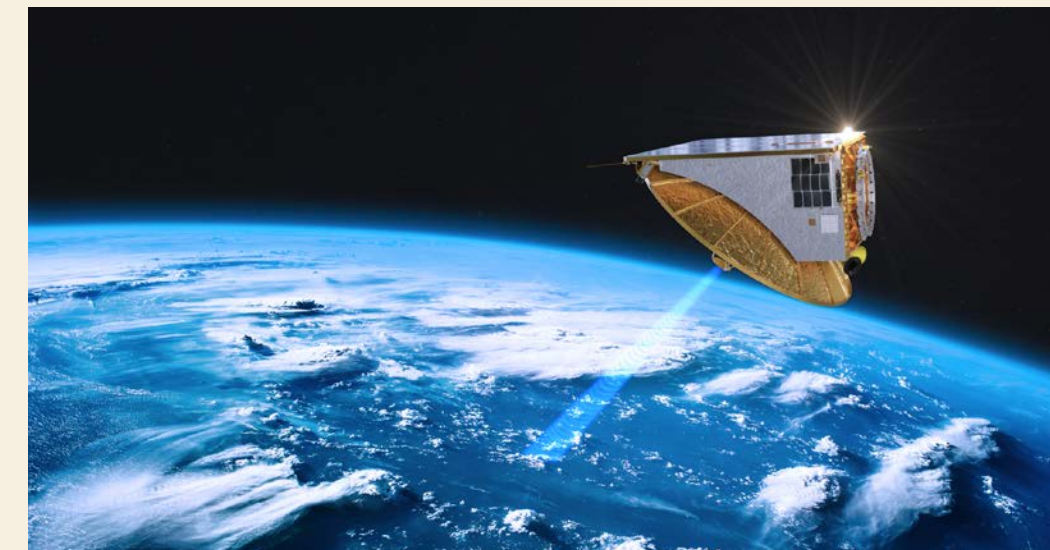
An illustration of Tomorrow.io's Resilience-series satellite. The Tomorrow.io Resilience Platform aims to utilize a constellation of more than 30 small satellites to provide near-realtime weather observations. The first satellite was launched in April 2023. Credit: Tomorrow.io
