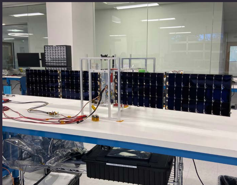
▼ The Arcstone spacecraft with solar panels installed as it is tested before being integrated for launch. Credit: Blue Canyon Technologies
