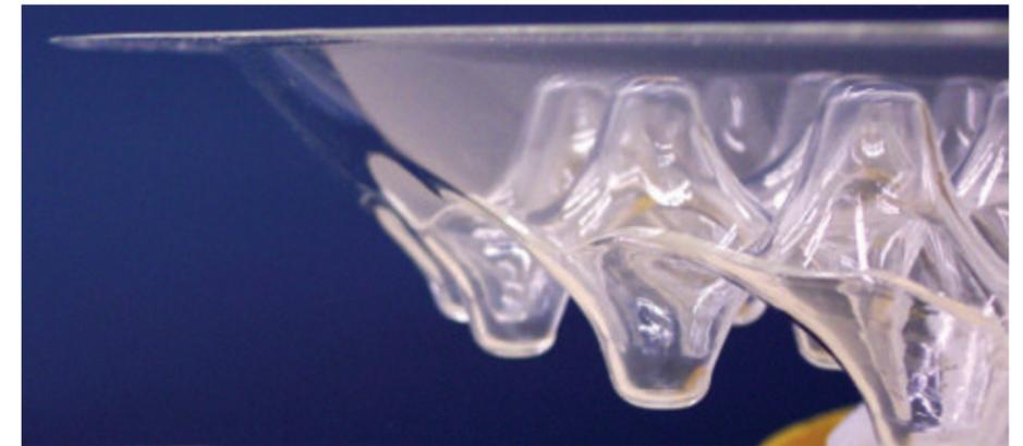
*in months to years and millions of dollars. This ACT project (PI: R. Egerman, ITT Geospatial Systems) demonstrated a new approach to mirror fabrication using borosilicate, an inexpensive and easy-to-work glass to develop new mirror designs.*
