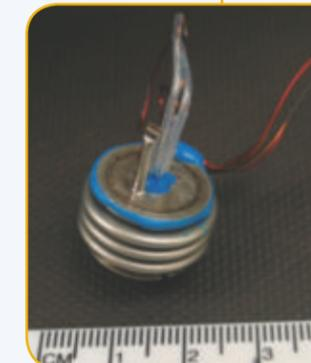
The CLARREO mission proposes to use phase change reference standards (melt cells) to recalibrate its on-board temperature sensors; but these cells have never been tested in space. In 2011, this project will conduct Thermal Phase Change Cell Demonstrations Onboard the International Space Station (ISS) and achieve in-space testing of two melt cell designs. (PI: M. Mlynczak, NASA LaRC)
