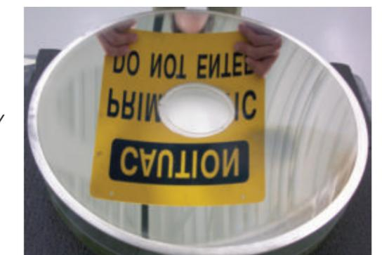
*Above, one of the 0.5m mirrors shown with a spray-silver coating after final polishing and ion figuring. (All images courtesy ITT Geospatial Systems)*
