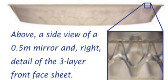
*Above, a side view of a 0.5m mirror and, right, detail of the 3-layer front face sheet.*
