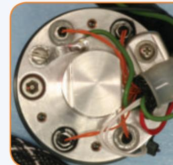
The **Advanced Accuracy Satellite Instrumentation for the CLARREO Mission** project seeks to develop and test several key calibration subsystems, such as temperature calibration for the blackbody cavity shown at left, dual absolute radiance interferometers, and an emissivity module. (PI: H. Revercomb, University of Wisconsin)
