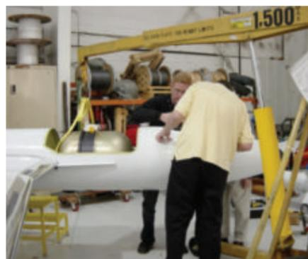
Above, one of the two INFLAME instruments is mounted in the wing tip tank of the Learjet aircraft. (Image courtesy Marty Mlynczak)
