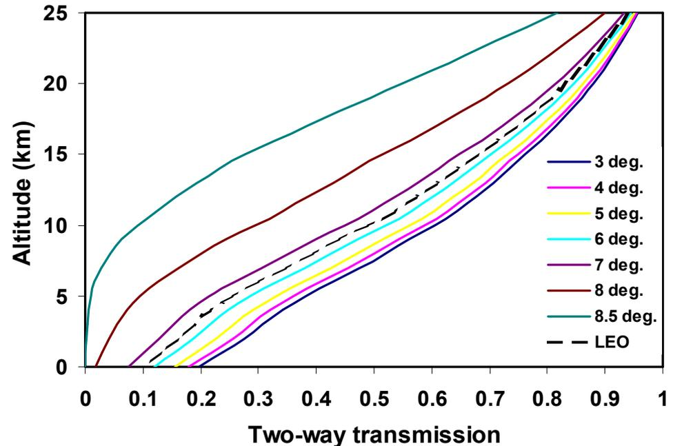
The sample plot is for a 355 nm wavelength using the NMP\* reference atmospheres.
