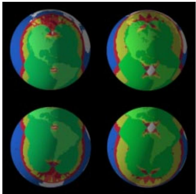
Fig. 1. Coverage map,  $50^\circ$  inclination on the left,  $65^\circ$  inclination on the right. Green indicates 3-d mapping, yellow 2-d and red 1-d mapping.
