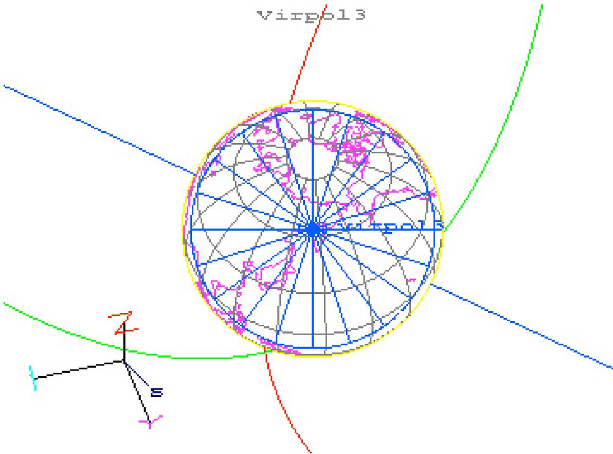
Figure 2. Down looking view from Virpol 3 (Blue—refer to Figure 1) with a FOV footprint directly over the Kamchatka Peninsula of the Russian Far East. The VPGS view from Molniya orbit is superior to that from the equatorial geostationary perspective (e.g., GOES, GMS, METEOSAT).
