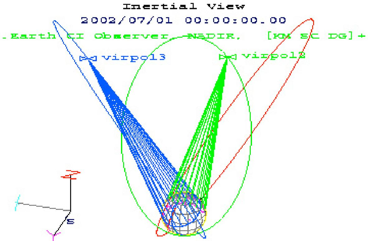
Figure 1: PVGS Orbital Tracks. Blue (Virpol 3) and Green (Virpol 2) are simultaneously covering the Earth's northern hemisphere, while Red (Virpol 1) is near perigee over the Antarctic. Apogee is at approximately 40,000km. The orbital period is 12hrs. (courtesy Dr. Ted Sweetser, JPL).
