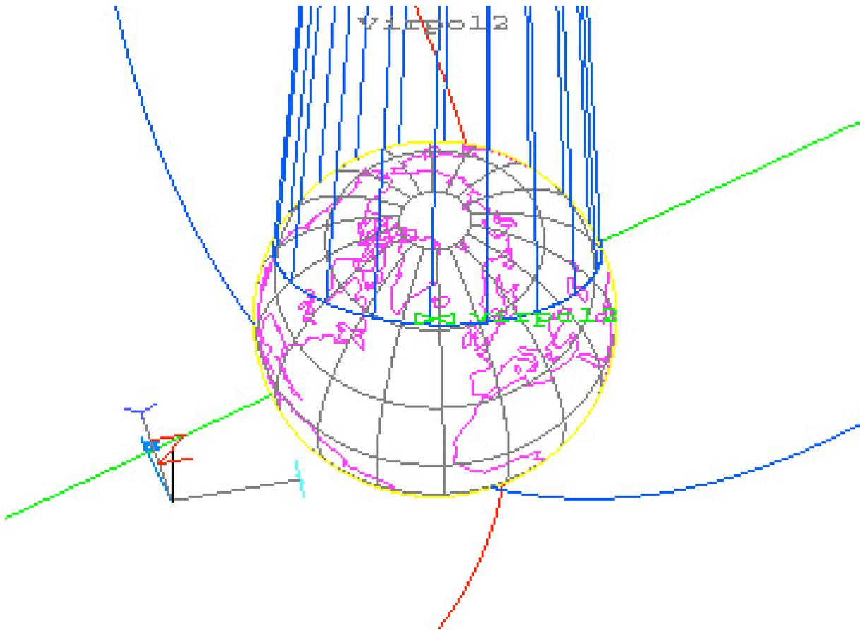
Figure 3. Down looking view from Virpol 2 (Green) of the North Atlantic with the center of the spacecraft FOV over Iceland. Notice the simultaneous coverage from Virpol 3 (Blue—refer to Figure 2).
