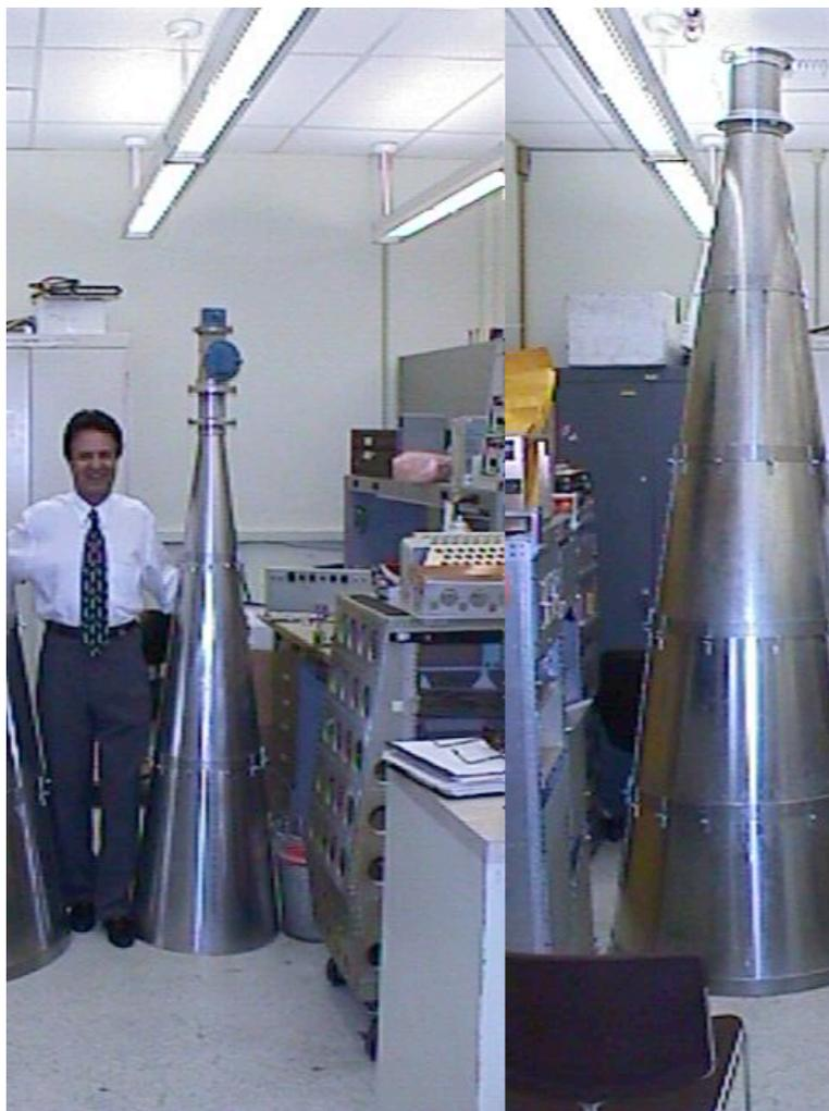
Figure 7: L- and S-band conical horn antennas, with Dr. Rahmat-Samii.
