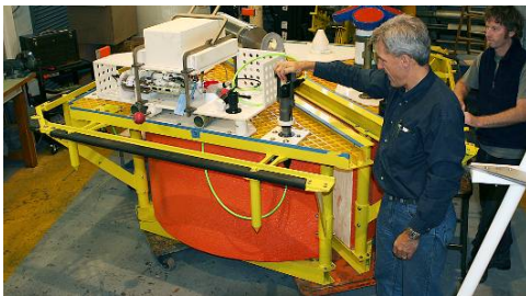
Figure 4: The subsurface float and secondary node, with instrument package and an Acoustic Doppler Current Profiler (ADCP).
