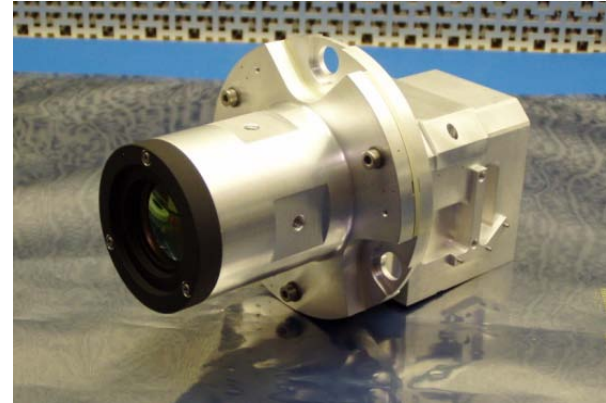
SWIR telescope and relays
