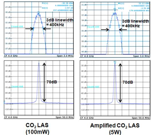
Fig. 6. Images showing <400kHz frequency uncertainty maintenance between reference laser and offset-locked laser (before and after fiber amplification). De-convolved amplifier output linewidth ~ 275 kHz.
