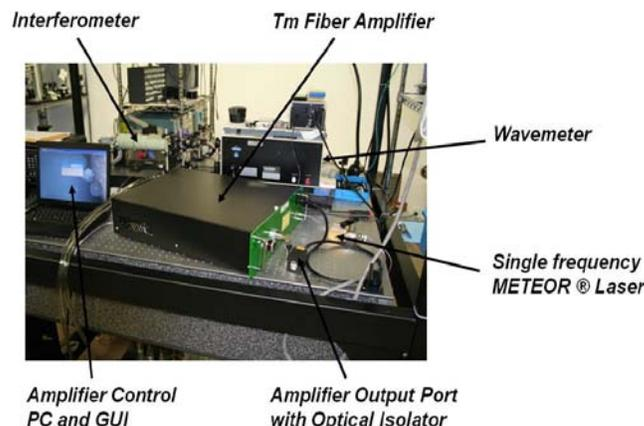
Fig. 2. Amplifier Test Configuration using Stand-Alone METEOR® Laser
