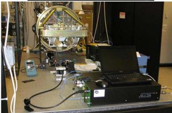
Fig. 3. Amplifier Test Configuration using CO<sub>2</sub> LAS Instrument
