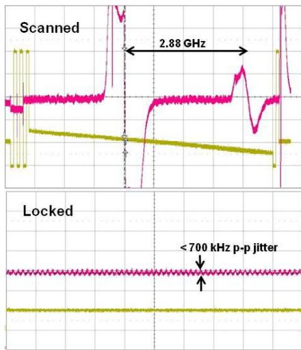
Fig. 5. Images showing < 700kHz frequency uncertainty maintenance of CO<sub>2</sub> LAS reference laser.
