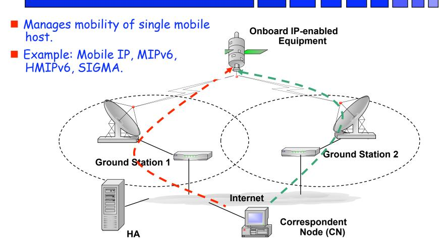
Satellite with IP-enabled equipment acts as mobile host / network.
