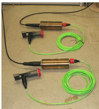
Fig. 3: ROV-mateable connectors and the electro-optical converters (in beryllium copper pressure cases) attached to each end of the (black) seafloor cable.
