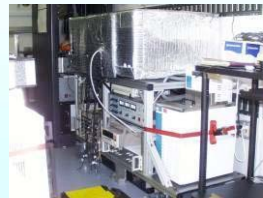
Receiver mounted in GLOW lidar for field tests and measurements
