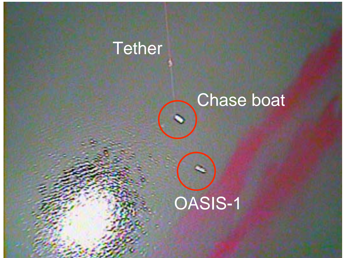
View from aerostat: chase boat, OASIS-1 and rhodamine dye
