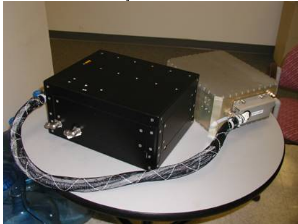
Figure 2 - Single frequency 355 nm Nd:YAG laser (gold) and Laser electronics unit (black)
