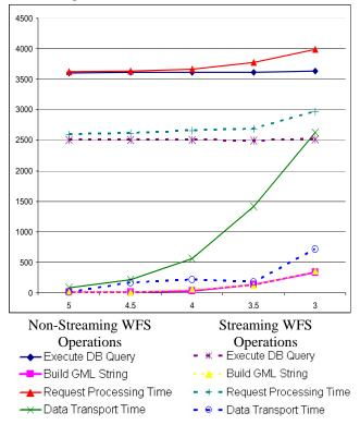
Fig. 1. Performance comparisons of the streaming and non-streaming WFS implementations showing the advantage of streaming the data over a messaging broker.
