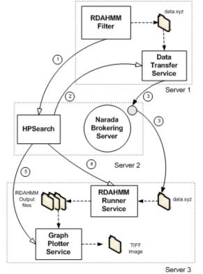
Fig. 3. System Architecture diagram for coupling RDAHMM with real-time GPS messages.
