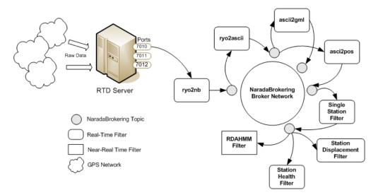
Fig. 2. Real-Time GPS messages are processed and served using various filters connected via NaradaBrokering messaging substrate.
