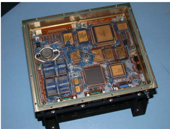
Fig. 2. The AIM module before integration into the FedSat satellite.
