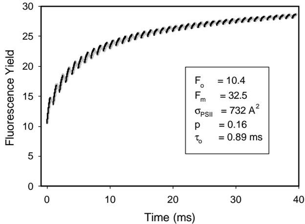
**Fig. 2** Typical fluorescence transient measured remotely at B2C in cottonwood trees, exposed to 1200 ppm CO<sub>2</sub> concentration. Black dots: experimental data points; grey line: numerical fit to a model described by (1-4), with photosynthetic parameters as shown in the inset.
