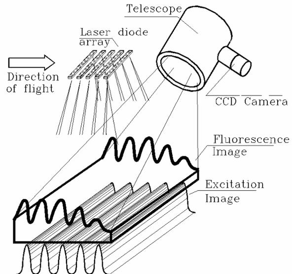
**Fig. 4** Airborne implementation of the LIFT method. The excitation signal, in a form of several stripes, is produced by an array of laser diodes. The excitation pattern, traveling at the speed of the airplane along the flight path, subjects the ground target to a temporally-modulated excitation signal, similar to that shown in Fig. 1. The resulting fluorescence image is collected by a 250 mm telescope, and acquired by a CCD camera.
