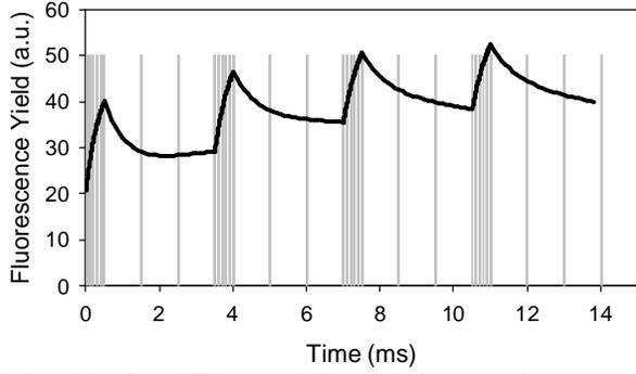
**Fig. 1.** Principle of the LIFT method. The excitation power is modulated by changing the frequency of the excitation flashes (grey bars). The fluorescence signal (black line) transiently increases when the excitation power exceeds the capacity of the photosynthetic electron transport, and decreases at low excitation power. The average excitation power is kept at about  $30 \text{ W/m}^2$  to satisfy ANSI Z-136.1 guidelines regarding eye-safe laser radiation.
