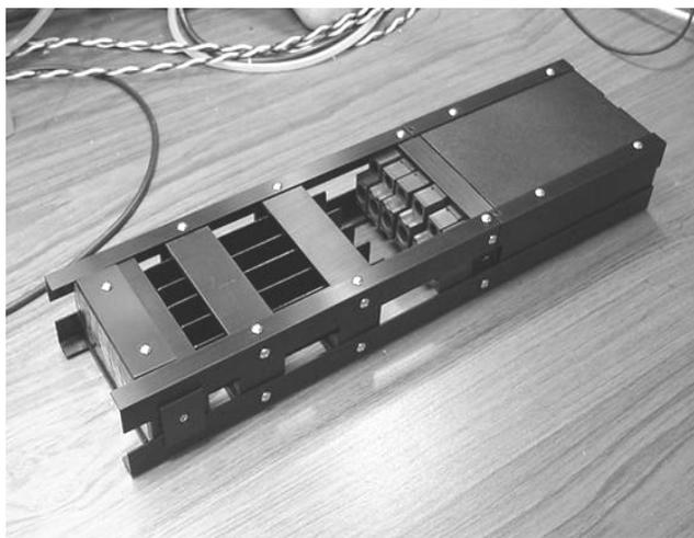
**Fig. 6.** Laser module with six laser diodes. Twelve of such modules are used in the airborne LIFT instrument.
