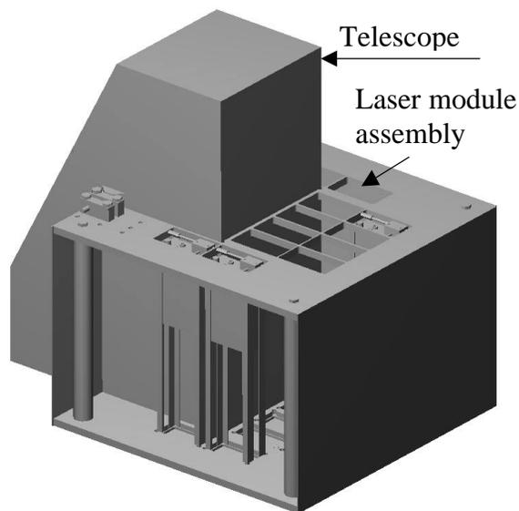
**Fig. 5.** Mechanical design of the excitation source and the emission telescope in the airborne version of the LIFT instrument.
