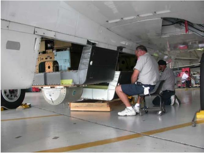
Figure 2. PSR undergoing installation on the WB-57.
